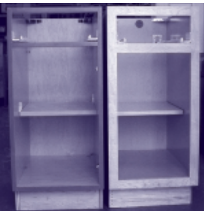
Frameless cabinets, left vs. face frame cabinets, right. Frameless cabinets always use full overlay doors; whereas with face frame cabinets there is a choice of inset, full overlay or partial overlay doors.
